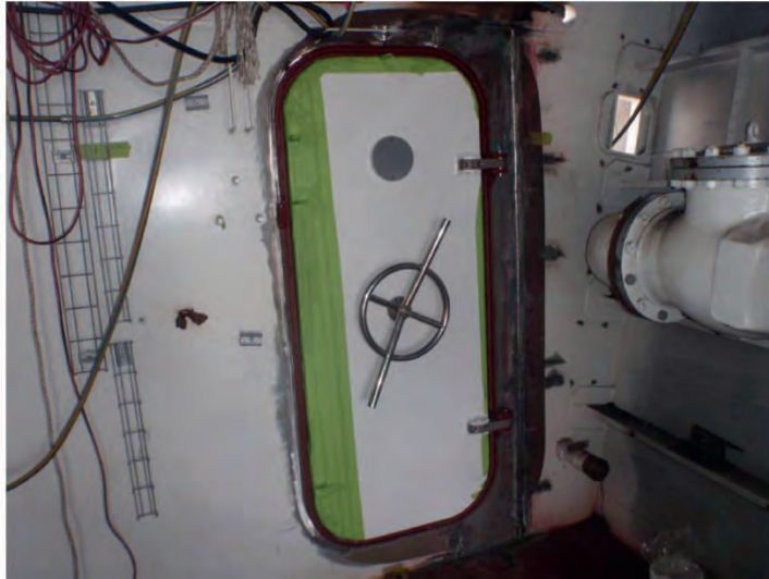
Figure 6.9: Rework on doorways to provide a minimum 90-degree opening
