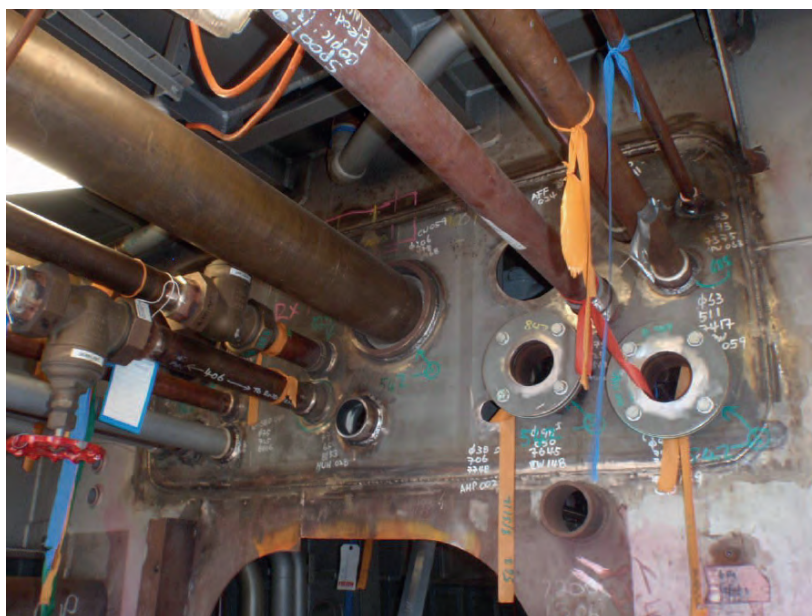
Figure 6.8: Piping system rework—Block 407 after block consolidation
