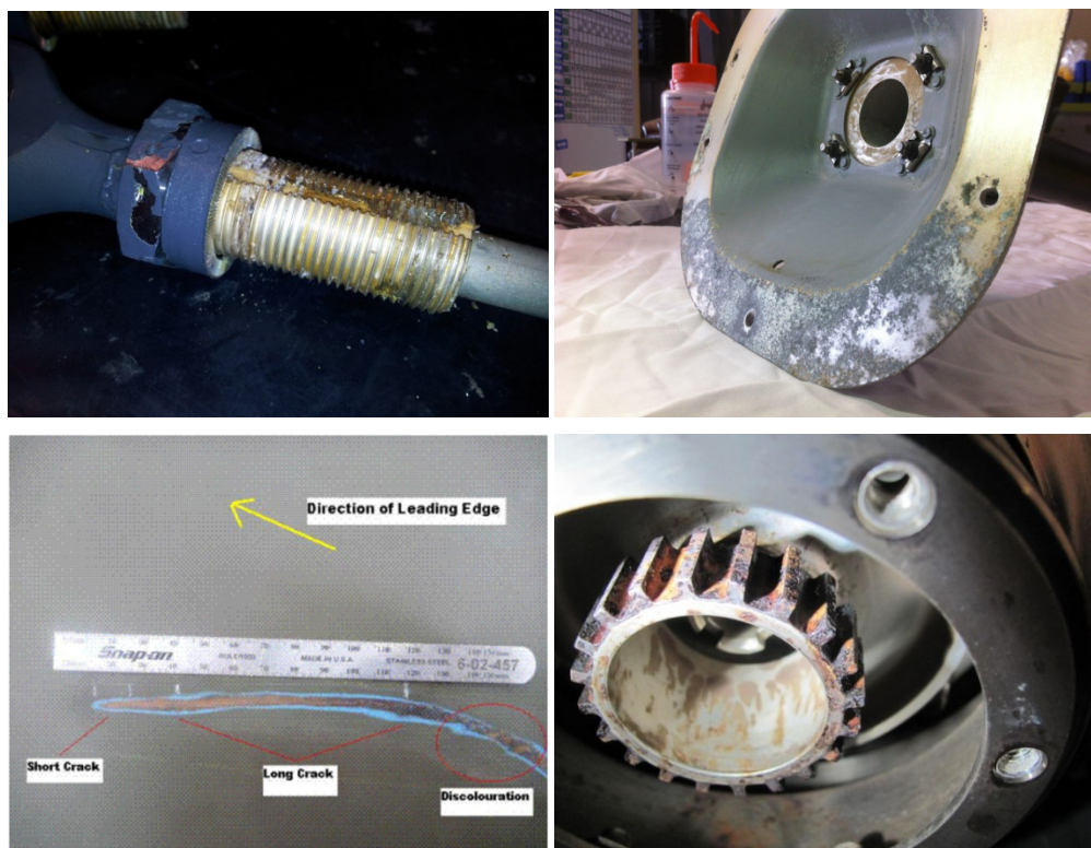
Figure 3.7: MRH90 aircraft corrosion and delamination
