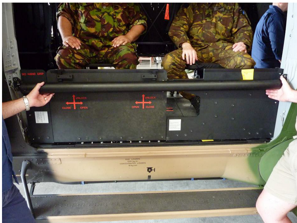
Figure 3.4: Sniper bar incompatibility with ballistic protection
