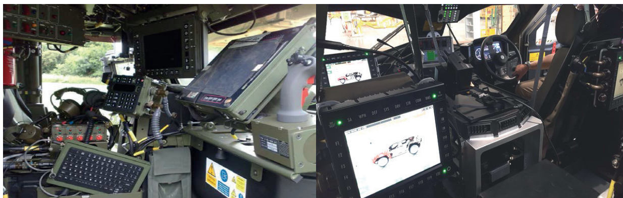
Figure 5.1: A vehicle cab before and after the Integral Computing System
