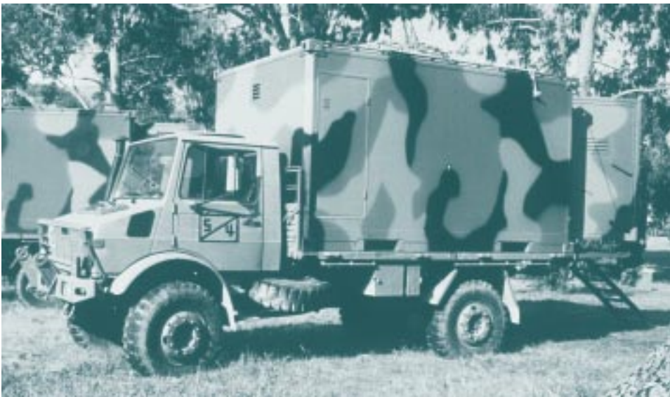
Unimog Medium (4 tonne) Truck with Workshop Shelter
