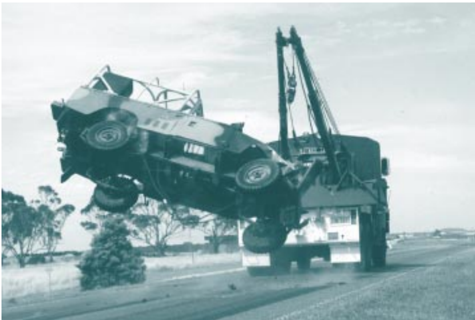
Mack Wrecker being used in the testing of the Perentie rollover cage
