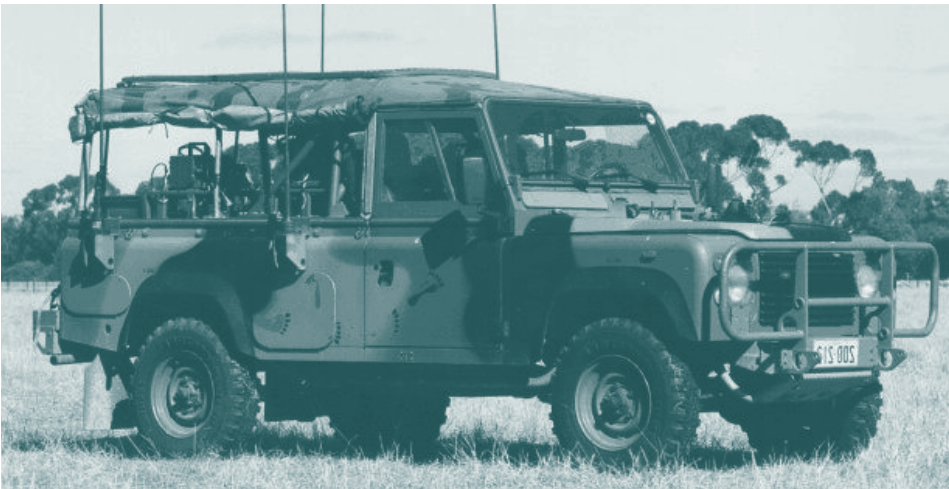
Land Rover Perentie Lightweight Truck Fitted For Radio
