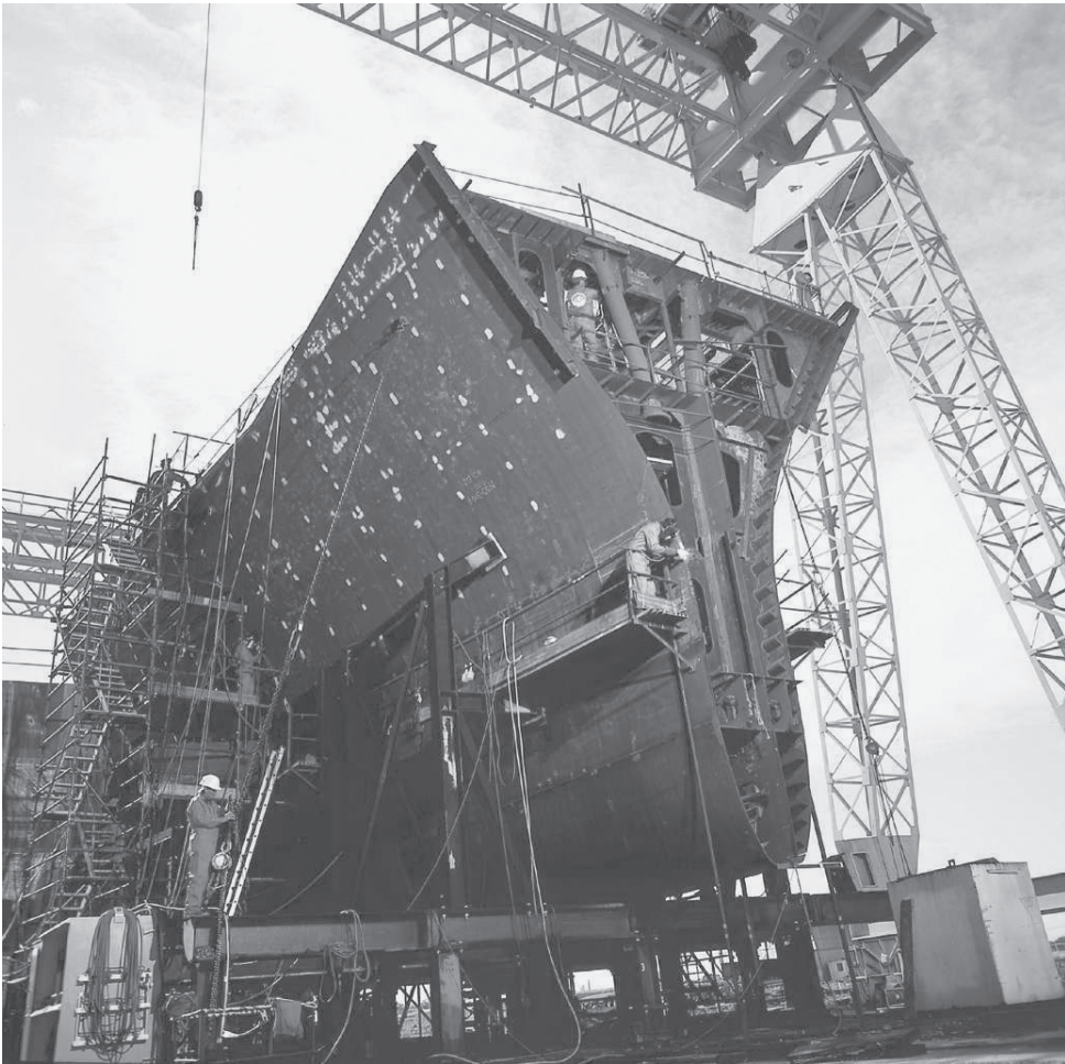
Construction of Anzac-class frigate, Forward module. Photo courtesy of Forgacs Shipyard Pty Ltd, Tomago NSW.
